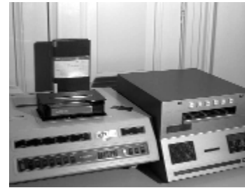
Cleaning machines for videotapes and preservation setup at the Netherlands Media Art Institute.
